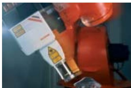
Hardening of a printing machine part with high power diode laser
