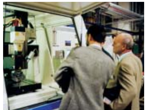
Demonstration of a hardening machine with an integrated high power diode laser in the laser hall of IWS during the workshop "Applications of High Power Diode Lasers"
