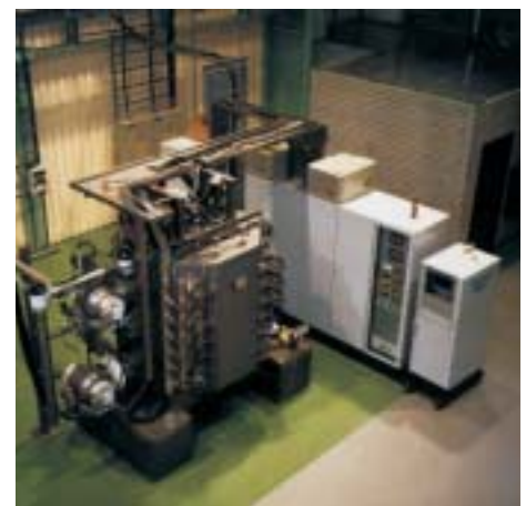
Laser-Arco ® - the technology to deposit Diamor ®
