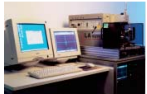
Laser-Acoustic measurement station for the non-destructive determination of thin film properties, acknowledged through the "R&D 100 Award 2001" in the USA
