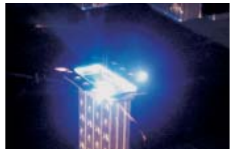
Welding of the tube / base plate joint of an exhaust gas heat exchanger utilizing a beam scanning optics
