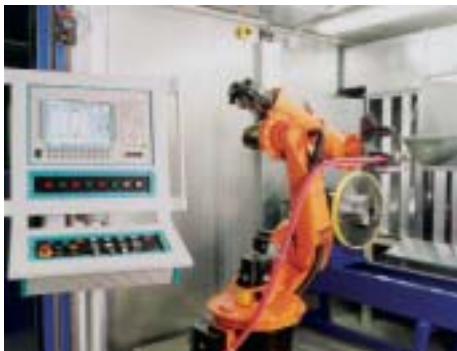
Atmospheric plasma spraying with laser coupling
